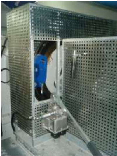
Close-up of the window in the brake disc protection for blocking the rotor.
